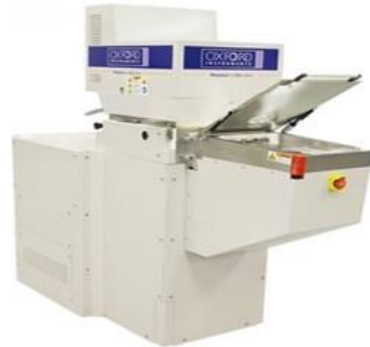
Oxford ICP Etcher with optical emission spectroscopy sensor
